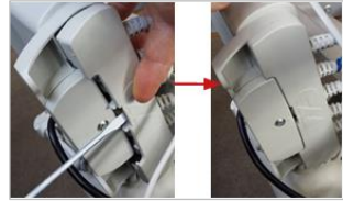
Fitting cable cover - Cable cover unclips/clips into place
